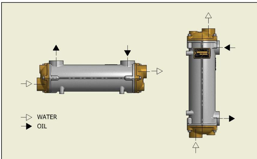
Multiple units can be connected in parallel:
