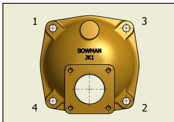
End covers must be refitted in the correct orientation to ensure correct performance.
